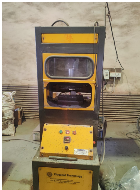
Photo-14.1: Photograph showing core splitter used to split borehole core
